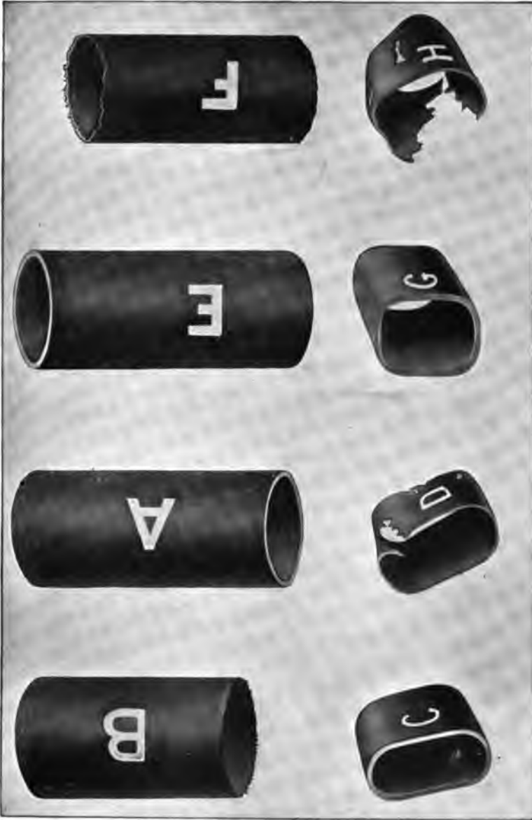
Fig. 19.—Corrosion of Steel Tubes. (From Paper by Albert Ladd Colby, A. S. Nav. Arch'ts, 1903.)
